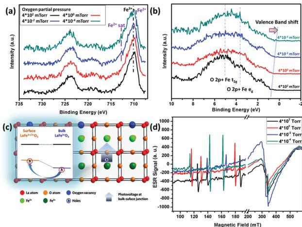
Fig. 1 Characterization of LFO films annealed under different oxygen pressures. (a) Binding energy of Fe 2p. (b) Normalized valence band spectra. (c) Band structure of the bulk–surface heterojunction. (d) Electron paramagnetic resonance spectra.
