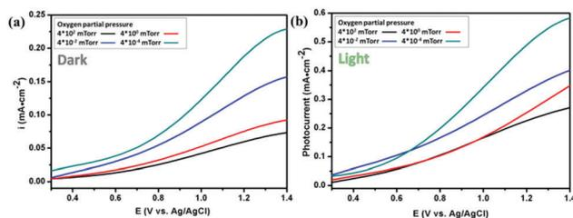
**Fig. 3** (a) Dark current, (b) photocurrent of OER in 0.1 M KOH for LFO films annealed under different oxygen pressures.
