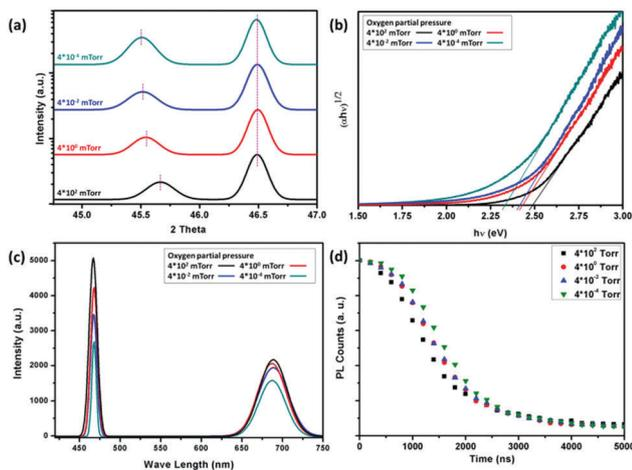
**Fig. 2** (a) High-resolution XRD patterns for LFO films annealed under different oxygen pressures with unchanged substrates STO (002). The slight down-shift of the epi-peaks of LFO (004) means lattice expansion. (b) Optical absorbance spectra have been converted into the form of the Kubelka–Munk function to show the absorption edge shift. (c) Photoluminescence spectra with an excitation wavelength of 290 nm. (d) Photoluminescence lifetime at an emission wavelength of 466 nm.
